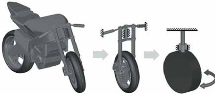
Fig. 1. A concept of the equivalent model used for the testing of numerical procedures
